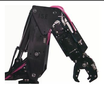
The *Magnum-6 Mini*, from the magnum family, is a rugged 6-function manipulator used primarily in ROV applications. This manipulator is designed to be reliable while operating in harsh environments. Components and assembly make this arm completely field serviceable.
